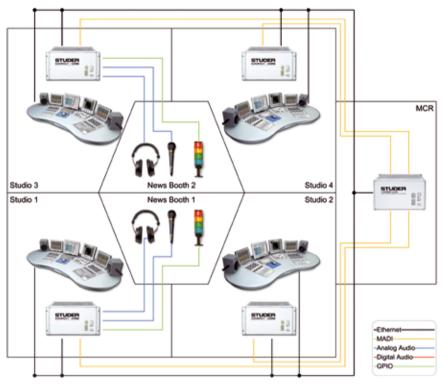
signal from Booth 2, while Booth I is at the same time used for the news with Studio I. The setup also allows a very flexible emergency switch-over, since every studio can connect to any voice booth.
